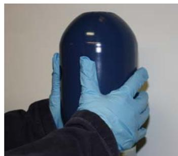
5. Screw cylinder cap in place by hand
