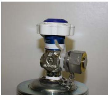
2. Use plastic tie or metal wire to secure valve handle in closed position
