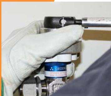
1. Tighten valve closed using specified torque
